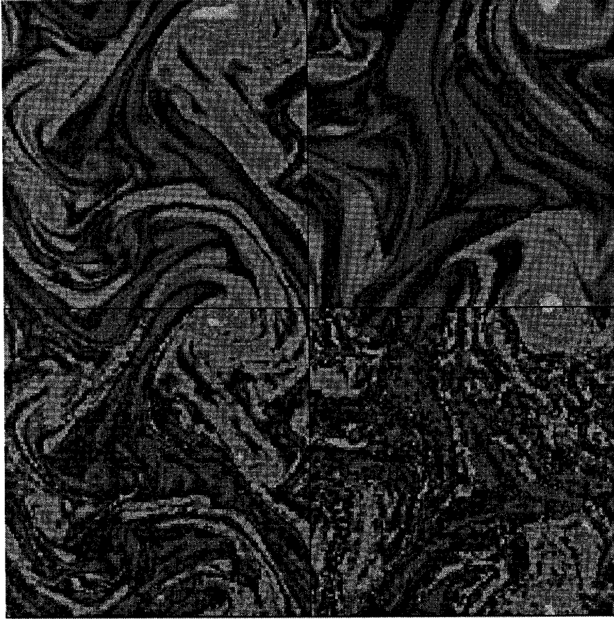
FIG. 1. Vorticity values at t = 20 and t = 60 for a pure Euler scheme (bottom pictures) and the eddy viscosity model (top pictures).
